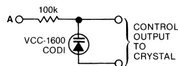
**FIGURE 8.** Stable quartz-crystal oscillators can operate with a single active device (a). You can achieve maximum frequency stability by mounting the oscillator in an oven and using a temperature-controlling circuit (b). A varactor network (c) can also accomplish crystal fine tuning. Here, the varactor replaces the oven and retunes the crystal by changing its load capacitances.
