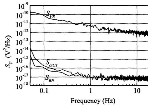
Fig. 4. Power spectral densities at the output of the new programmable voltage reference ( $S_{OUT}$ ) together with the DA converter output noise ( $S_{VR}$ ) and the preamplifier background noise ( $S_{BN}$ ).
