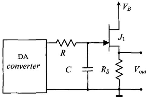
Fig. 1. A simplified schematic of a filter and circuit for the realization of a low noise programmable voltage reference.
