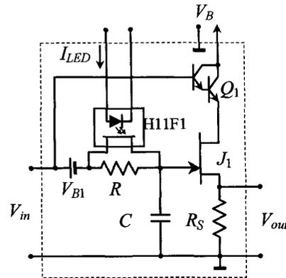
Fig. 2. Actual filter and buffer circuit used in the new programmable voltage reference.
