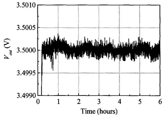
Fig. 6. Detail of the output voltage value as measured by the high resolution AD converter that is part of the control loop (Fig. 3).
