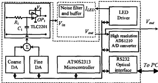
Fig. 3. Block diagram of the entire system. The optical link is used to avoid EM interferences from the PC.
