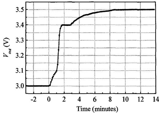
Fig. 5. Output voltage transient response of the new programmable voltage reference after a set point change occurring at  $t=0$ s.
