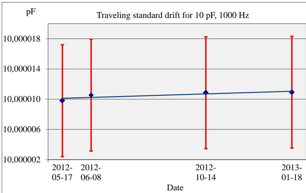
Figure 1 Behaviour of the travelling standard for 10 pF
