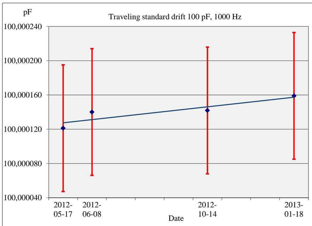
Figure 2 Behaviour of the travelling standard for 100 pF
