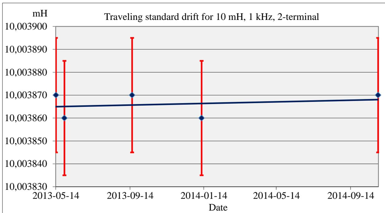
Figure 1 Behaviour of the travelling standard for 10 mH (2-terminal)
