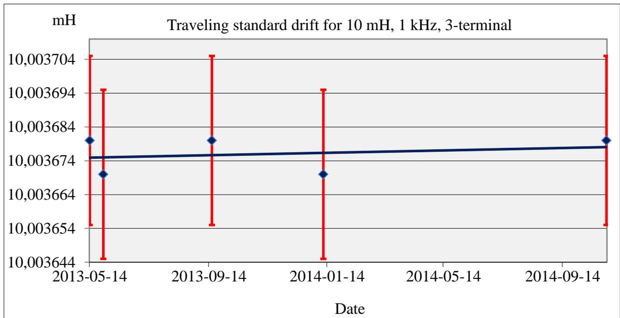
Figure 2 Behaviour of the travelling standard for 10 mH (3-terminal)
