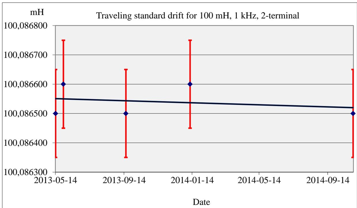
Figure 3 Behaviour of the travelling standard for 100 mH (2-terminal)
