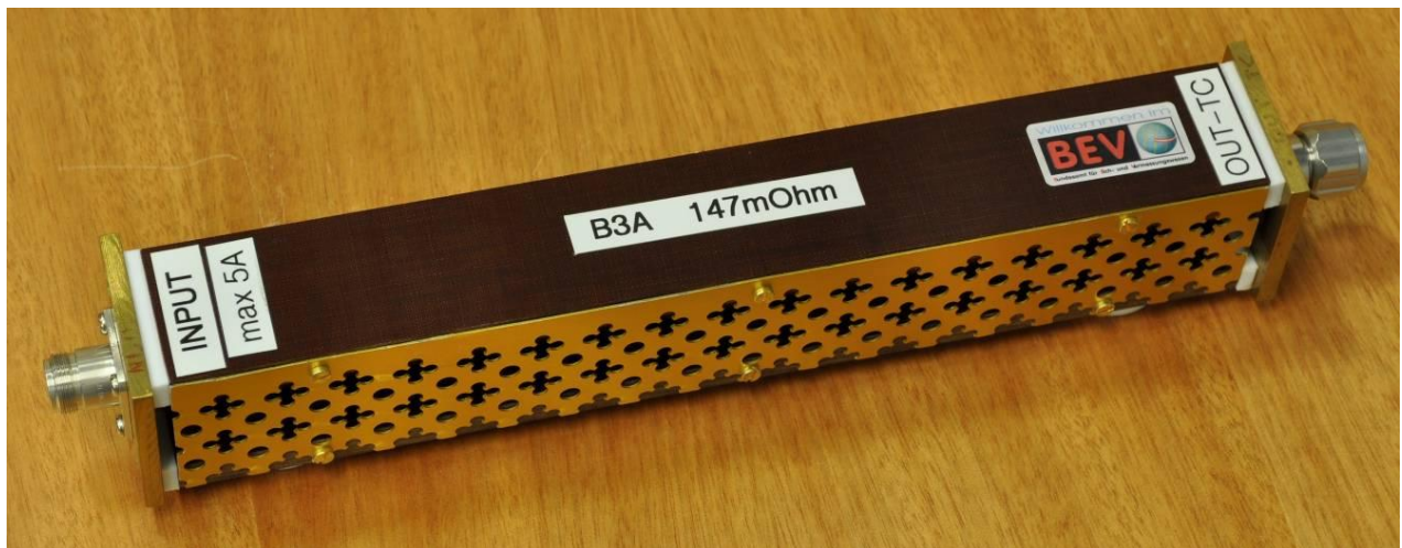
Figure 2: Physical layout of the 5 A travelling standard.
