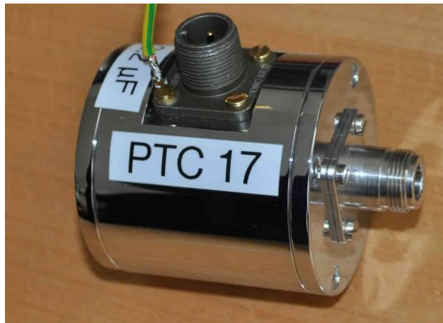
Figure 1: Physical layout of the 10 mA travelling standard.
