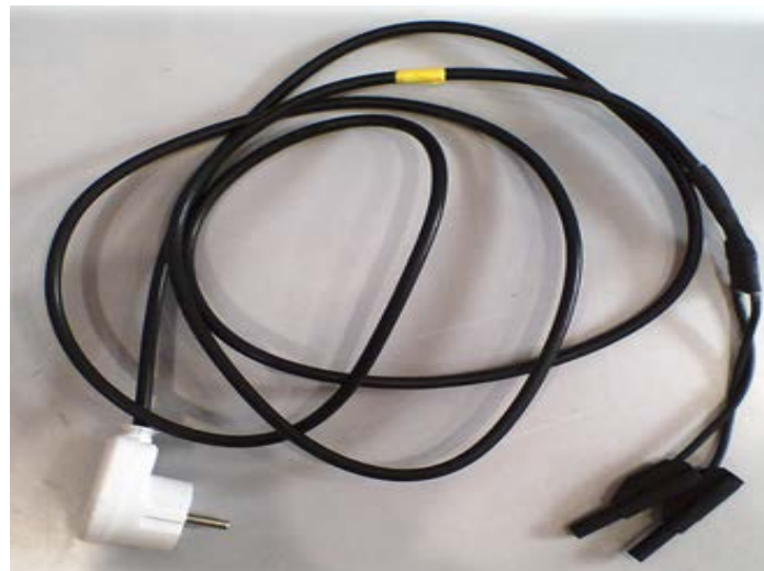
Figure 3 Power cable of travelling standard RD-33-332
