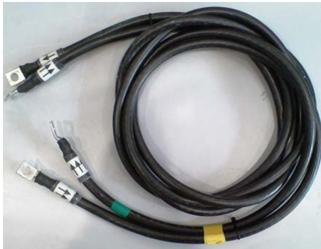
Figure 4 Current cables for connection travelling standard RD-33-332
