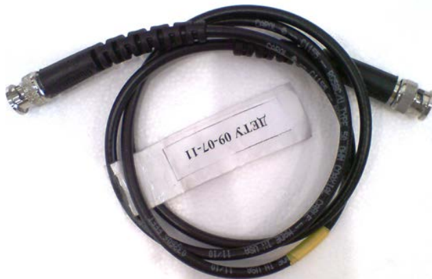
Figure 6 Pulse cable for connection travelling standard RD-33-332
