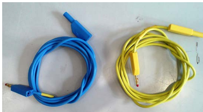
Figure 5 Voltage cables for connection travelling standard RD-33-332
