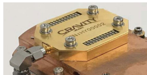
Fig. 5 NMIJ-fabricated two volt Josephson chip mounted on the cold plate
