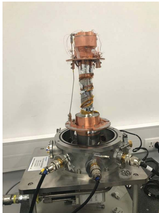
Fig. 3 Two-stage G-M cryocooler with NMIJ-fabricated Josephson chip mounted on the cold plate
