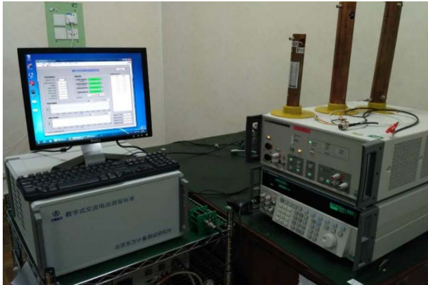
Figure 3. AC Current Digital Measurement System
