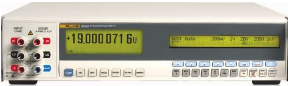
Figure 4. A Fluke 8508A DMM measures the outputs of the working resistance standards for transferring to the multifunction calibrator. Photo courtesy of Fluke.
