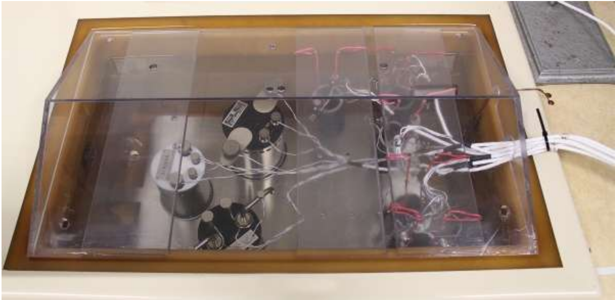
Figure 7. At the top of the resistance chain, Fluke reference resistors reside in oil baths for temperature stability.
