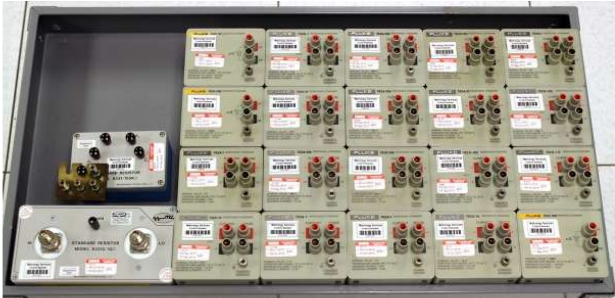
Figure 3. Fluke 742A resistance standards are used to check multifunction calibrators for resistance.
