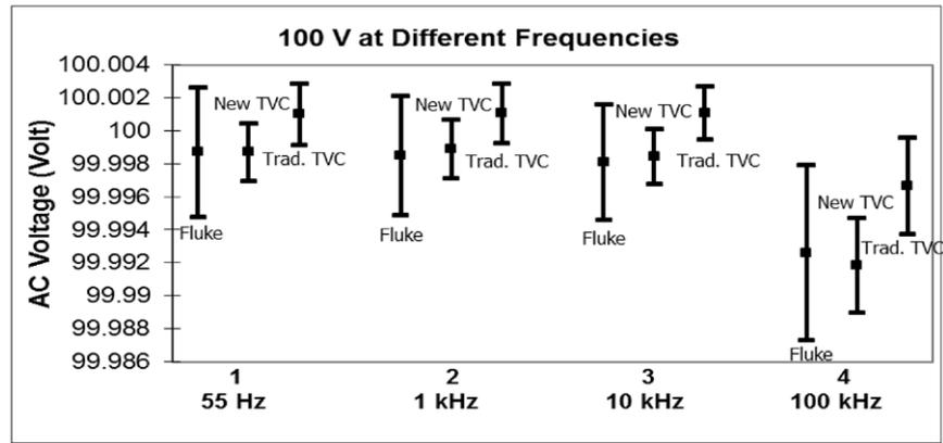
Figure 6. 100V ac voltage measurements at different frequencies.
