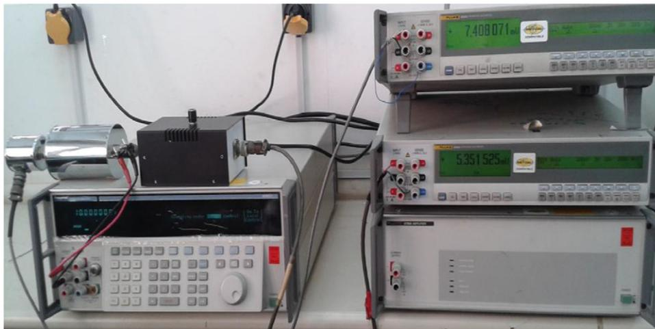
Figure 3. Automatic system for the new TVC calibration.
