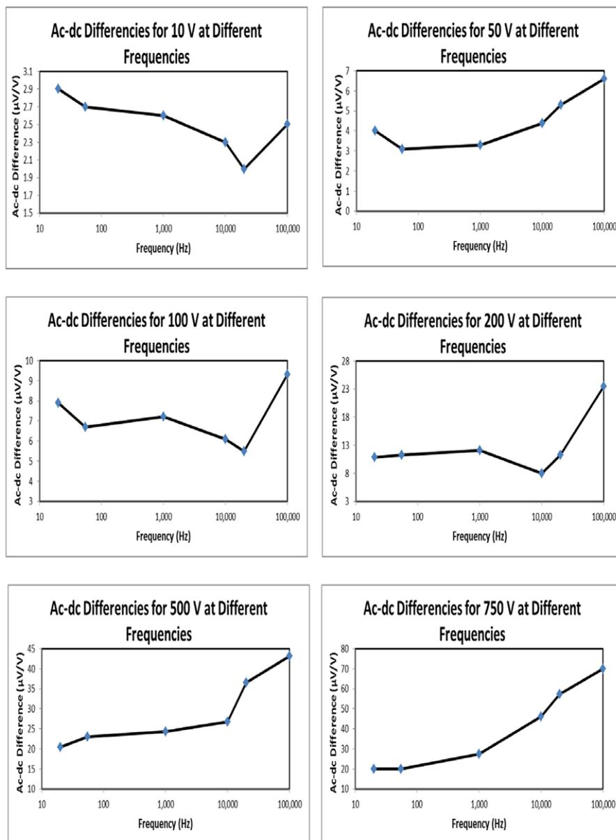
Figure 4.  $\delta_t$  for the new TVC at different voltage ranges and frequencies.
