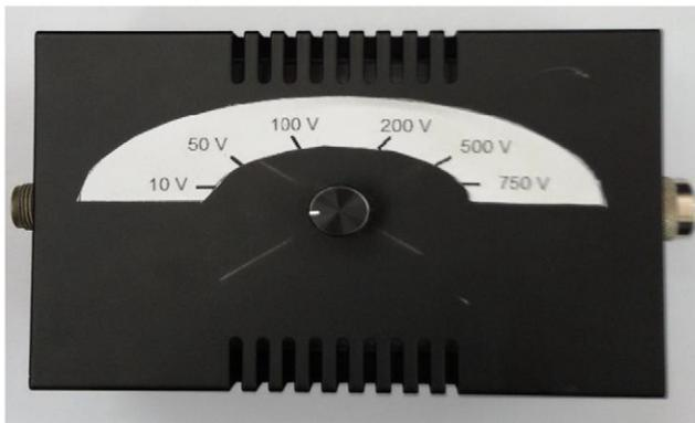
Figure 2. Implementation of the new range resistors by using a six-pin selector.
