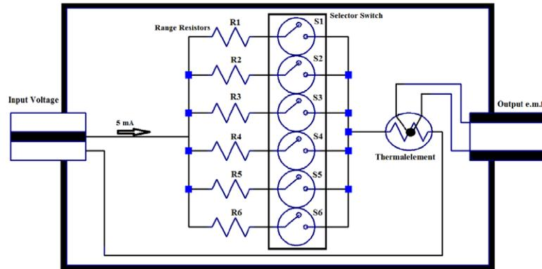
Figure 1. Construction of TVC with new multi-range internal range resistors.
