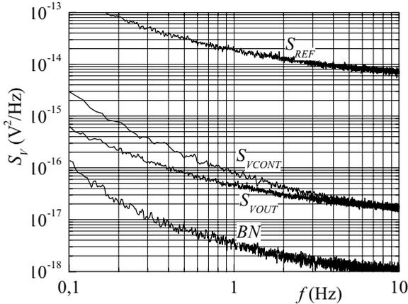
Fig. 7. Power spectral density of voltage fluctuations measured at the output of the circuit in Fig. 5 ( $S_{VCONT}$ ). The power spectrum  $S_{VOUT}$  of the voltage fluctuations at the output of the circuit in Fig. 1 is reported as a reference.
