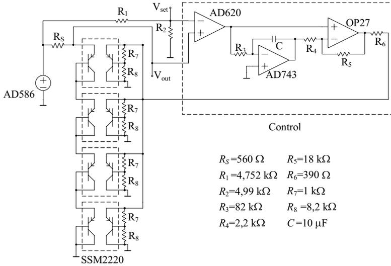
Fig. 5. Complete schematic of the low noise voltage reference including the temperature compensation system. The circuit within the dashed box acts as an error amplifier with a proportional-integral action. By changing the current supplied to the transistors used as heaters, the voltage  $V_{OUT}$  is made to approach the target voltage  $V_{SET}$ .
