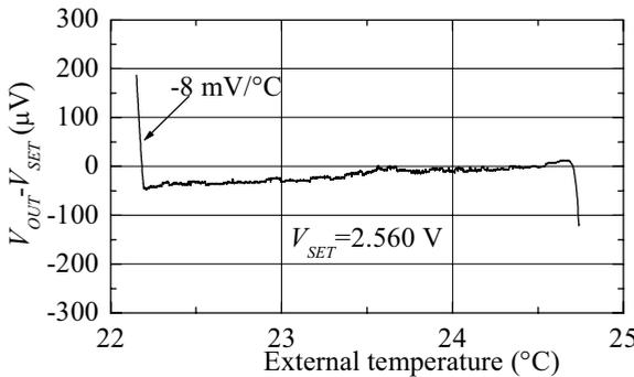
Fig. 6. Voltage error ( $V_{OUT} - V_{SET}$ ) at the output of the circuit in Fig. 5 versus external temperature. The temperature control system is active in the range from 22.2 to 24.8 °C. Outside this range the temperature control circuit is saturated and therefore the temperature coefficient of the voltage source is  $-2\text{N mV}/^\circ\text{C}$ .
