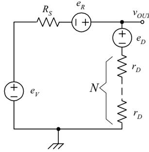
Fig. 3. Small signal equivalent circuit for the calculation of the output voltage noise. The equivalent noise source  $e_D$  accounts for the noise introduced by the  $N$  diodes as discussed in the text.
