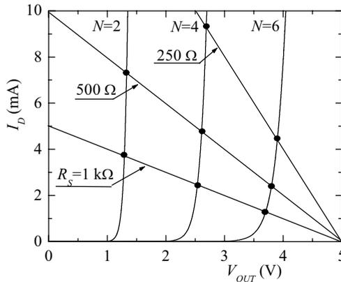
Fig. 2. Operating points for the circuit in Fig. 1 for a few values of  $N$  ( $N = 2, 4, 6$ ) and  $R_S$ . The curves representing the I-V characteristics of the series connected diodes (SSM2220) were obtained by direct measurement at room temperature. For drawing the load curve we assumed a voltage reference  $V_R = 5$  V.
