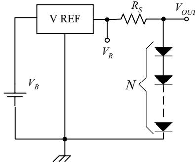
Fig. 1. A simple implementation of a low noise voltage reference. The number  $N$  of diodes connected in series together with the values of  $R_S$  and of the reference voltage  $V_R$  set the output voltage.
