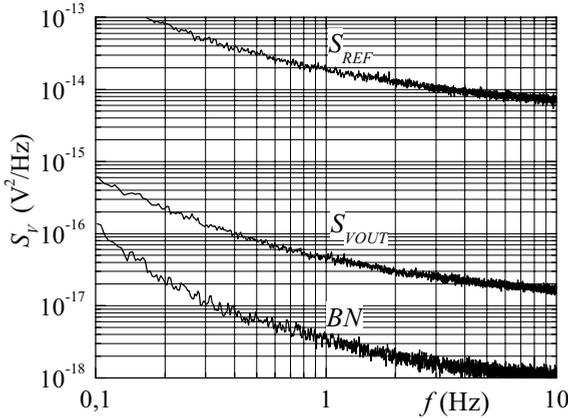
Fig. 4. Power spectral density of voltage fluctuations measured on the circuit in Fig. 1.  $S_{VOUT}$  is the spectrum of the voltage fluctuations at the output of the system;  $S_{REF}$  is the spectrum of the voltage noise at the output of the solid state voltage reference AD586,  $BN$  is the equivalent input noise of the ultra low noise amplifier employed for the measurements.
