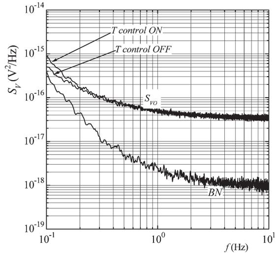
Fig. 11. Comparison between the output noise when the temperature control system is off (same as curve A in Fig. 9) and on. A slight increase in the noise can be observed at very low frequencies.
