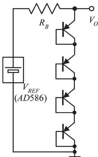
Fig. 1. Very simple low-noise voltage reference as proposed in [9].
