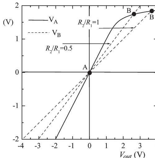
Fig. 4. Voltages  $V_A$  and  $V_B$  in the circuit of Fig. 3 as a function of the voltage  $V_O$  for different values of the ratio  $R_2/R_1$ . Two equilibrium points exist for each ratio  $R_2/R_1$ , labeled A and B in the figure.
