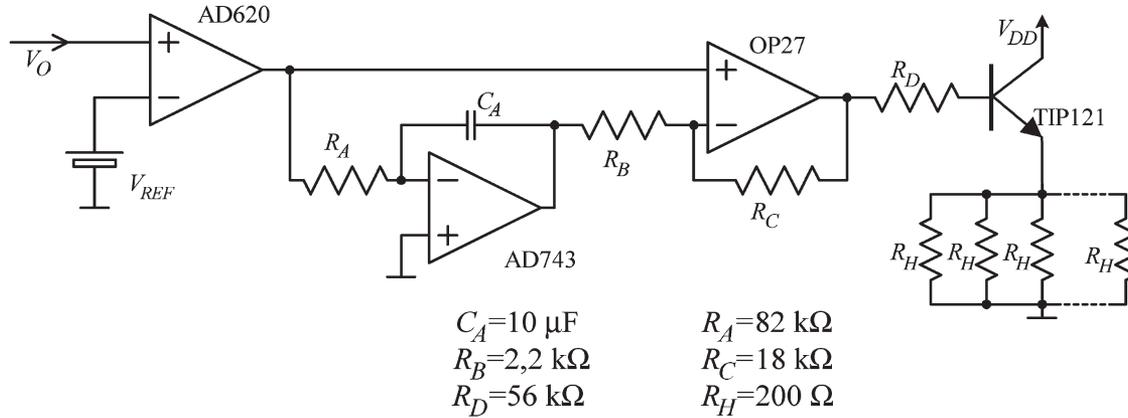
Fig. 7. Complete schematic of the temperature control system employed for reducing the temperature dependence of the output voltage of the new low-noise reference.
