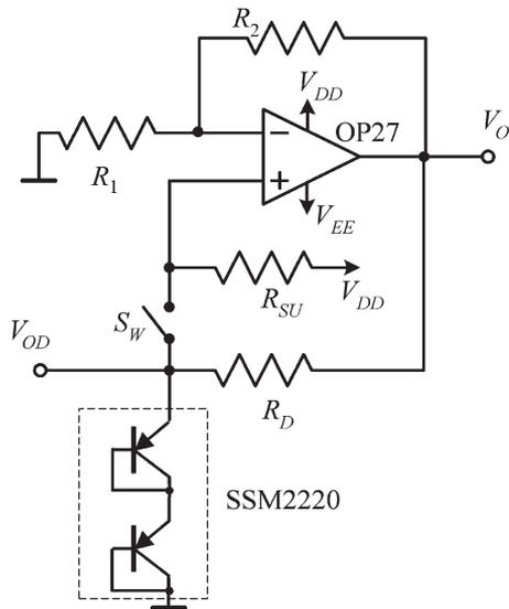
Fig. 8. Actual implementation of the new reference voltage. The presence of the high-value resistance  $R_{SU}$  together with the switch  $S_W$  allows bringing to operate in the proper equilibrium point at power on.
