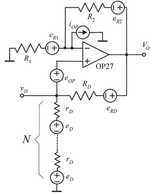
Fig. 5. Equivalent small-signal circuit for the evaluation of the output noise. All relevant noise sources are shown in the figure. Reprinted with permission from C. Ciofi, G. Scandurra, and G. Cannatà, "A new circuit topology for the realization of low noise voltage references", *Proceedings of the 20th International Conference on Noise and Fluctuations (ICNF 2009)*, Pisa, Italy, 14–19 June 2009, 599–602 Copyright 2009 American Institute of Physics.
