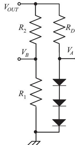
Fig. 3. Simplified circuit for calculating the equilibrium point of the circuit in Fig. 2 ( $N = 3$  is assumed).
