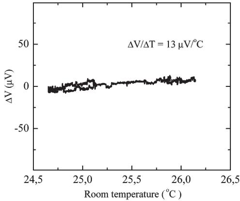
Fig. 10. Plot of the difference between the actual output voltage and the nominal voltage (5 V) as a function of the ambient temperature during one day of continuous operation of the voltage reference while the temperature control system was active.
