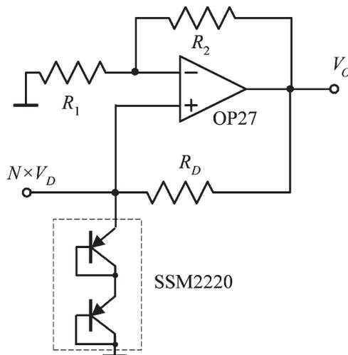
Fig. 2. Schematic of the new low-noise voltage reference. Reprinted with permission from C. Ciofi, G. Scandurra, and G. Cannatà, "A new circuit topology for the realization of low noise voltage references," *Proceedings of the 20th International Conference on Noise and Fluctuations (ICNF 2009)*, Pisa, Italy, 14–19 June 2009, 599–602 Copyright 2009 American Institute of Physics.
