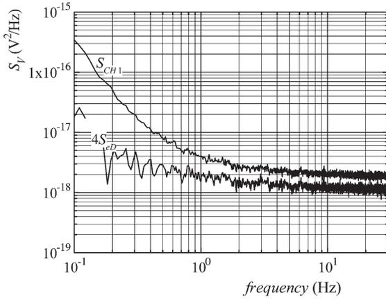
Fig. 6. Voltage noise across four diodes in series with a 1-mA bias current ( $4S_{eD}$ ). Cross correlation between the output of two low-noise amplifiers connected to the output of the system was used for estimating the noise produced by the diodes. The equivalent input noise of one of the amplifiers during measurement is shown in the figure ( $S_{CH1}$ ).
