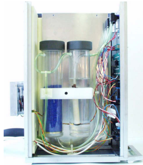
Fig. 6. Containers of the humidity conditioning of the air inside the enclosure.
