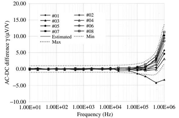
Fig. 5. AC–DC transfer differences of JSTC06 elements
