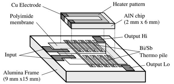
Fig. 1. Structure of JSTC06 thermal converter element
