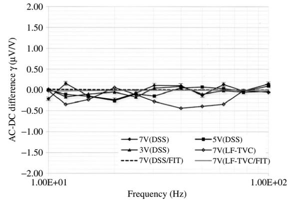
Fig. 3. Low-frequency characteristics of JSTC06 element
