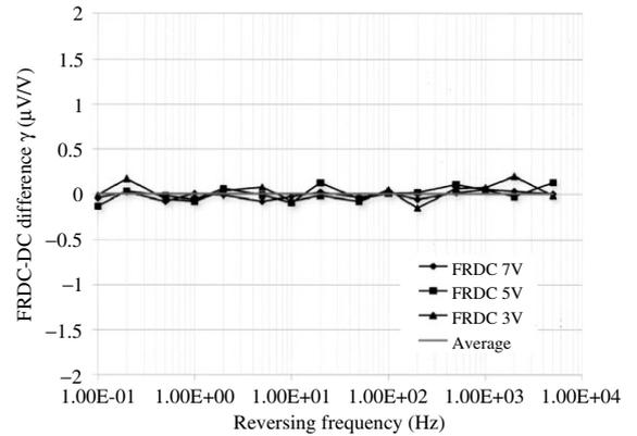
Fig. 2. FRDC-DC difference measurement of JSTC06 element
