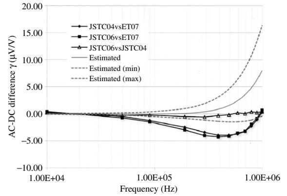
Fig. 4. High-frequency characteristics of JSTC06 element
