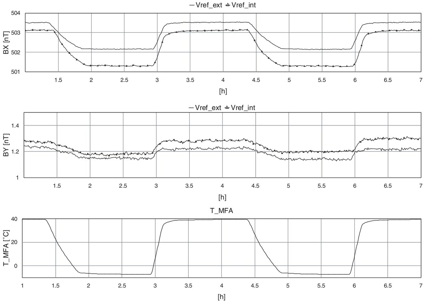
**Figure 14.** Gain drift of fluxgate channel X and offset drift of fluxgate channel Y with MFA temperature and external and internal voltage reference.
