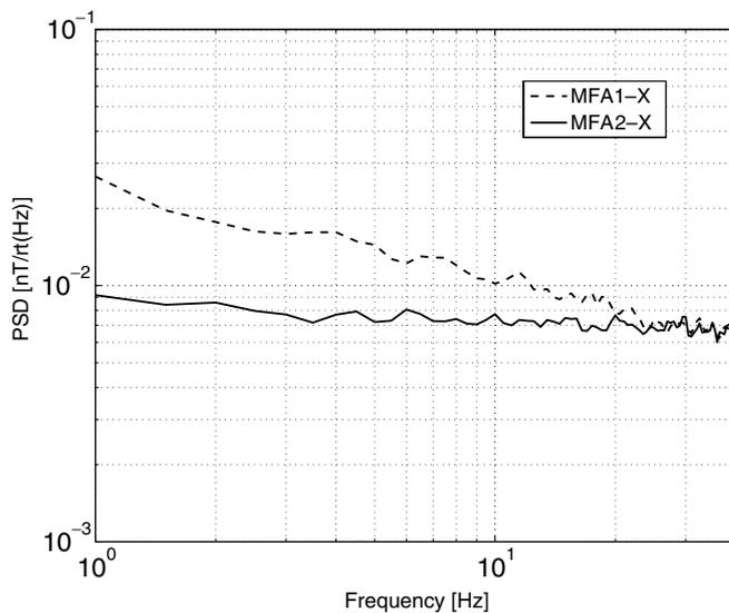
Figure 8. PSD of error cancellation output data from MFA-1 (without CDS) and MFA-2 (with CDS).
