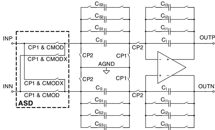
Figure 6. Switched capacitor integrator with an adjustable synchronous demodulator (ASD) and variable gain setting.
