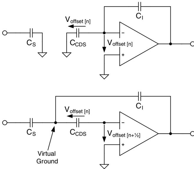
Figure 7. Principle of the correlated double sampling.
