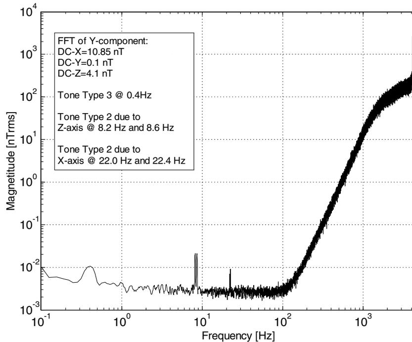
Figure 17. Spectrum of Y-channel error cancellation output with tones.
