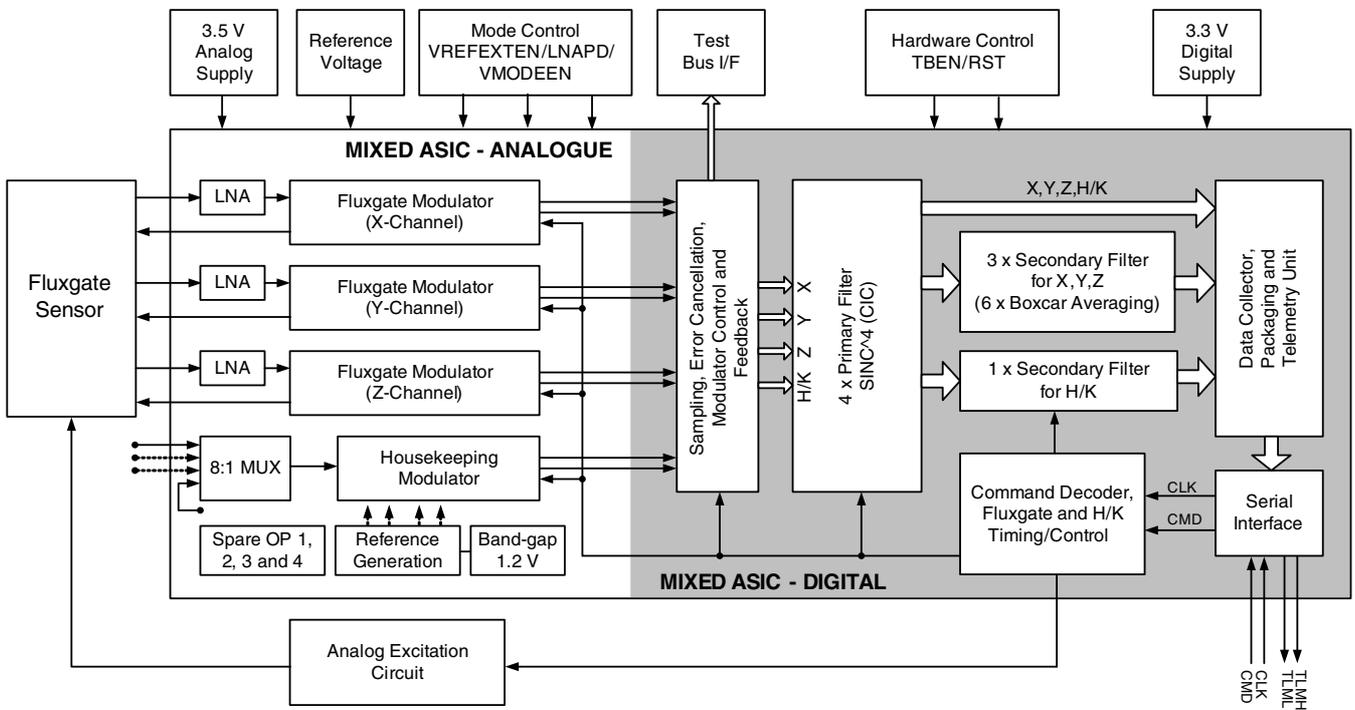
Figure 3. Block diagram of the redesigned magnetometer front-end ASIC.
