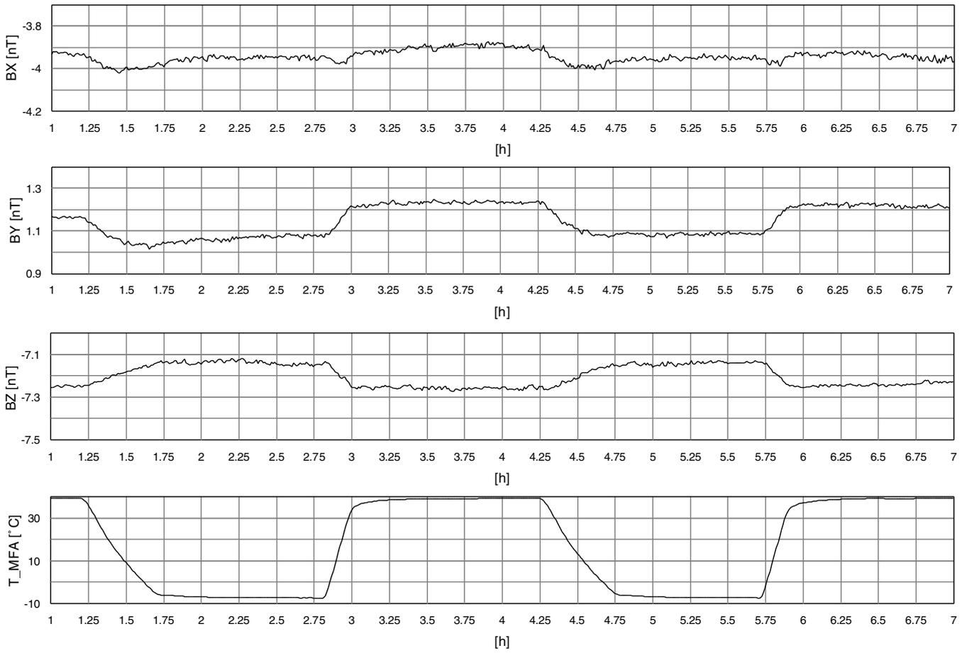
Figure 13. Offset drift of fluxgate channels with MFA temperature.
