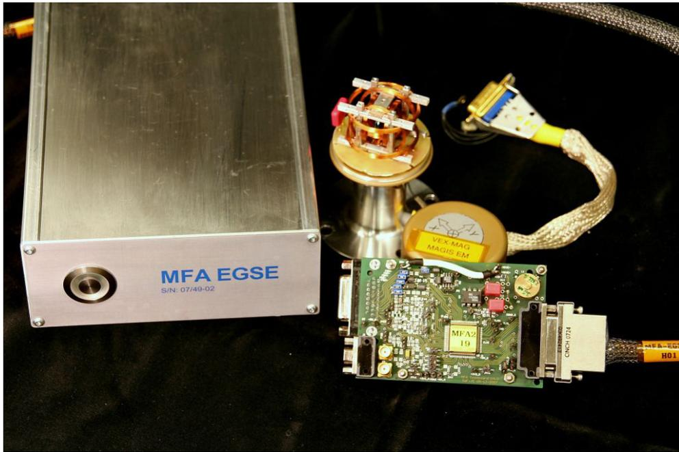
Figure 9. MFA test setup with a Venus Express sensor.
