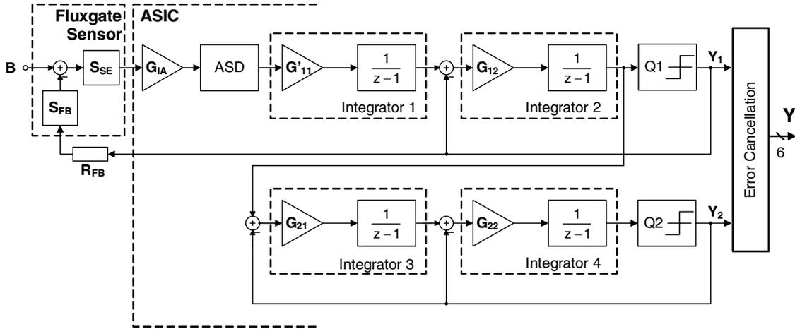
Figure 5. Linearized model of the modified 2–2 cascaded fluxgate modulator.
