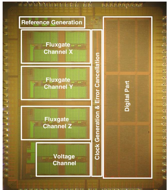
**Figure 1.** Chip micrograph of the magnetometer front-end ASIC (version 2).
