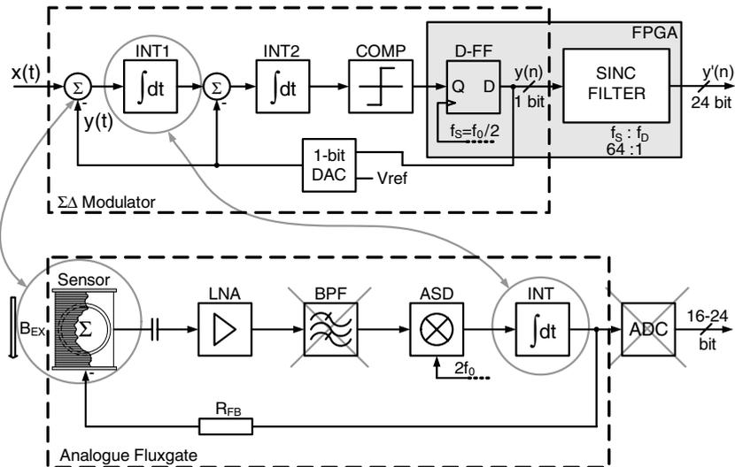
Figure 2. Merging of a second-order sigma-delta modulator with the fluxgate control loop.
