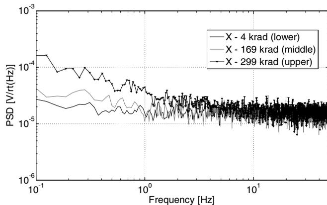
Figure 16. PSD plot of X-channel error cancellation output with short circuited input during irradiation.
