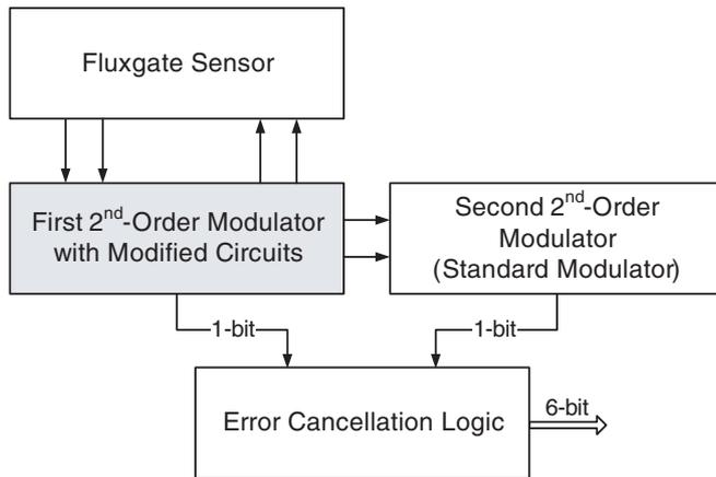
**Figure 4.** Block diagram of the 2–2 cascaded fluxgate modulator.
