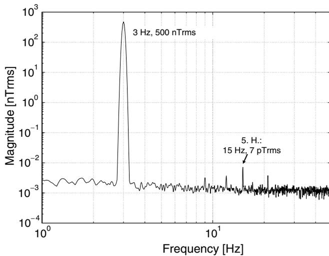
Figure 12. Total harmonic distortion.
