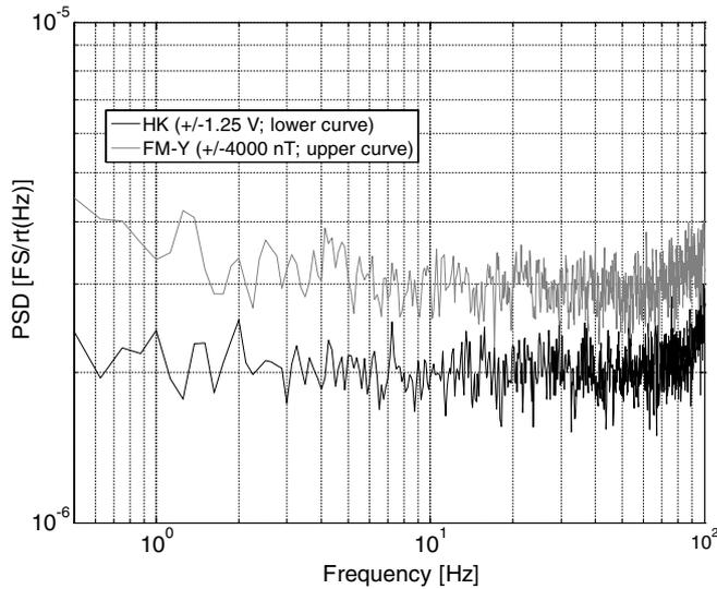
Figure 11. Comparison of the error cancellation output noise floor in field and voltage modes.
