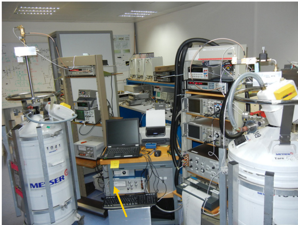
Figure 1. The new BIPM transportable JVS on the left-hand side and the BIPM primary standard operated since the first on-site direct comparison (right-hand side). Both JVS are connected directly together for comparison in the BIPM laboratories. The arrow shows the detector used to measure the voltage difference between the two JVSs.
