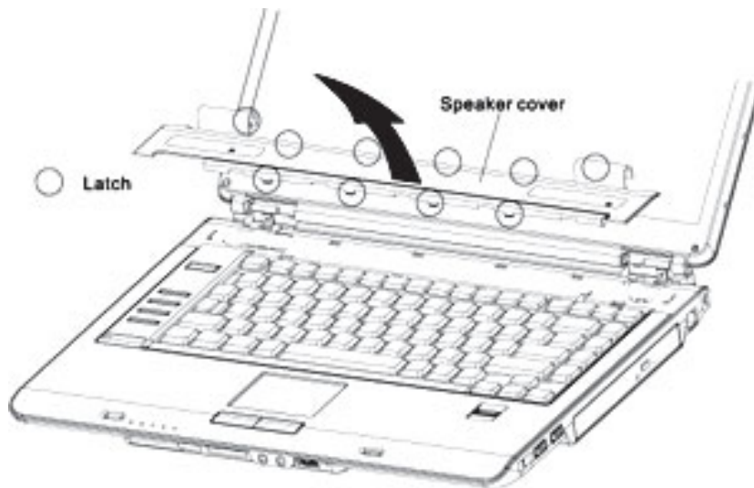
Figure 4-12 Removing the speaker cover
