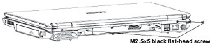
Figure 4-19 Removing the screws from the back of the computer
