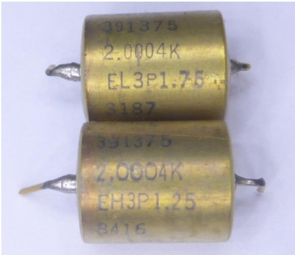
This kind of resistance was removed from the Fluke 731B voltage reference. The reason why it is said to be poor is because the resistance value is not exactly 2k, the temperature drift is 1.75 and the other 1.25 is relatively large, and it is positive, so it is not easy to compensate with copper resistance. If the NTC compensation of parameter B here is not used, it cannot be used as a standard resistor. 2. The parameter measurement circuit after testing two resistors in parallel is like this:
