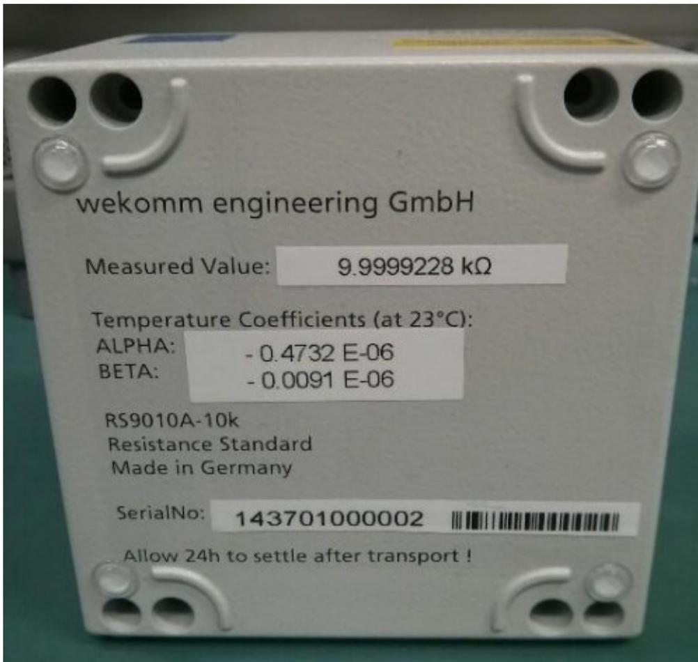
D=-7.72 (large enough) A=-0.4732 (not small) B=-0.0091 (very good) D and A are relatively large. The reason is that Wekomm adopts the doctrine when making this standard. The resistance core is A Vishay VHA518-7 gold-sealed metal foil resistor was led out intact without any correction or compensation.
