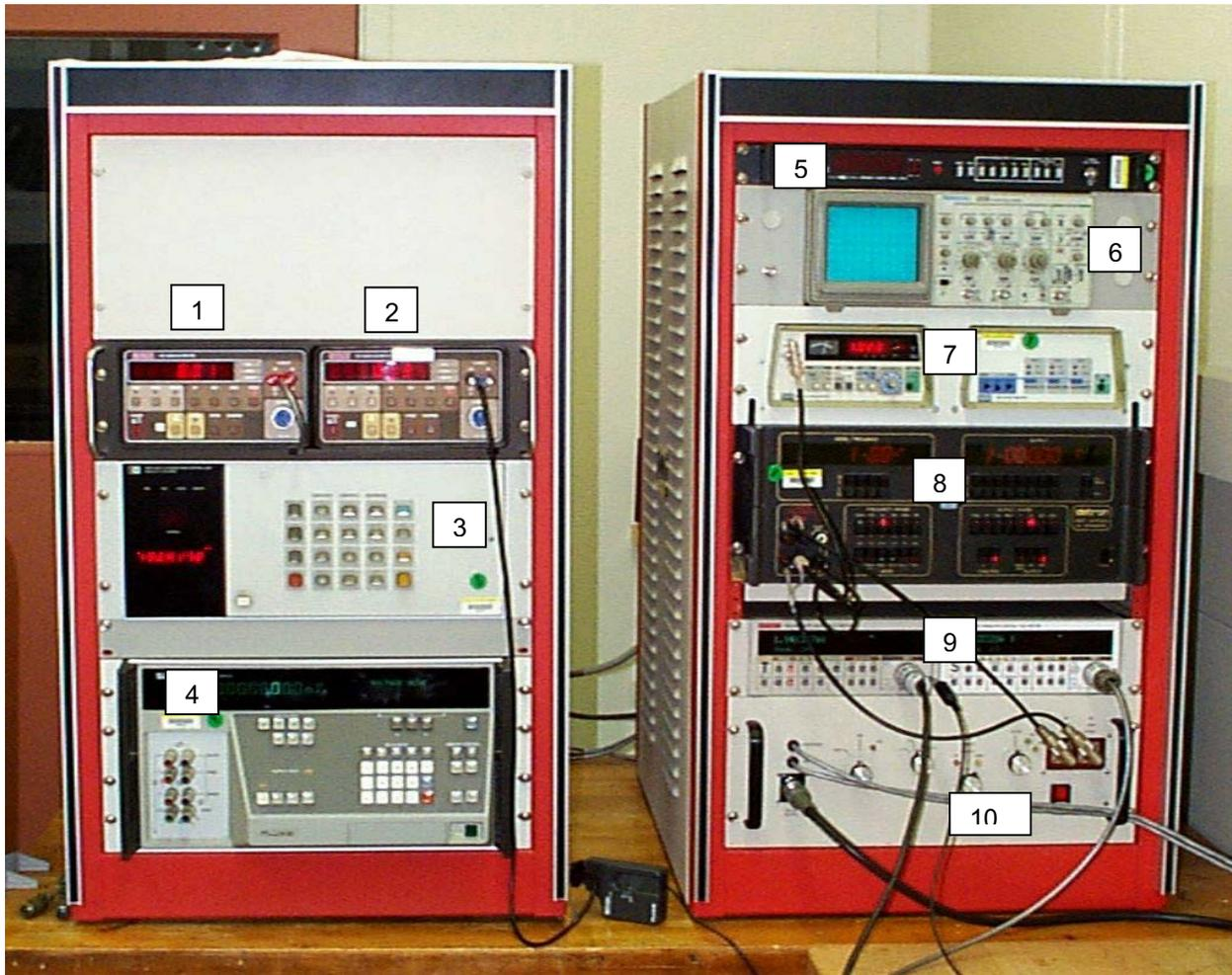
Figure 1. Photograph of NIST Automated System II. The other three automated systems are similar. The components of the system are shown in Table 1.
