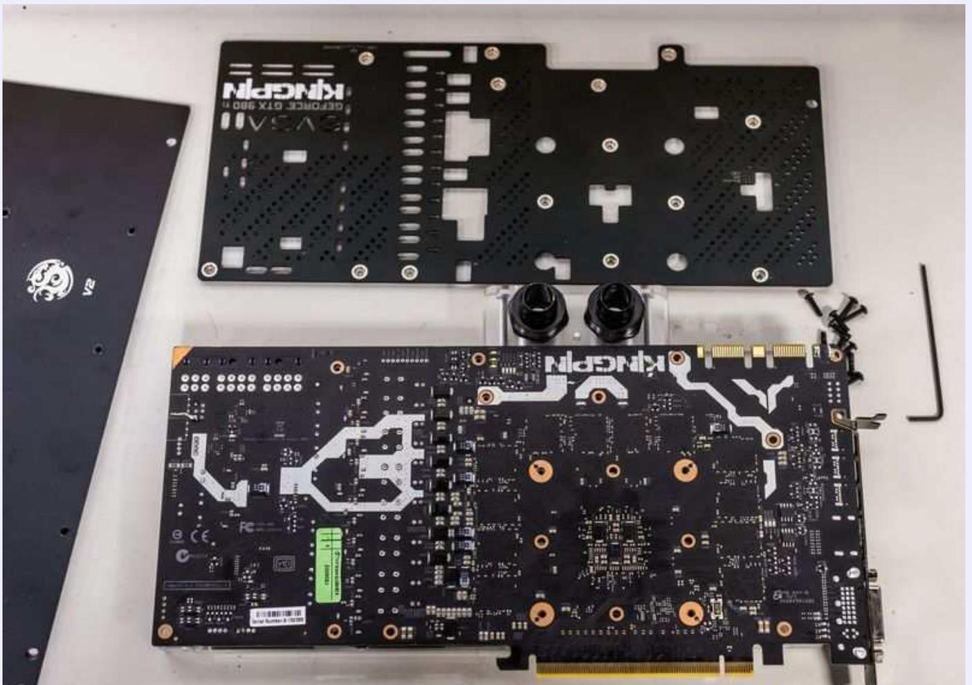
Installed block, front & back side
