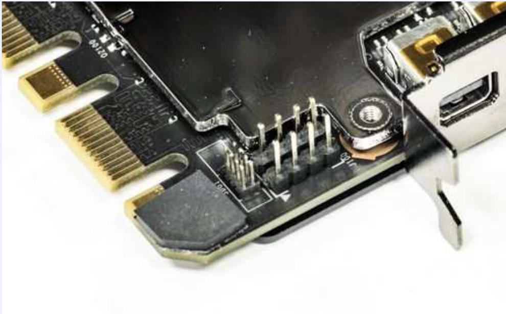
You have access to this port with both stock fansink operation and watercooling/LN2. Connect UART cable to VGA's serial port like this photo below. It could be little tricky to get cable between fansink cover, so use tweezers to fix cable in position.
