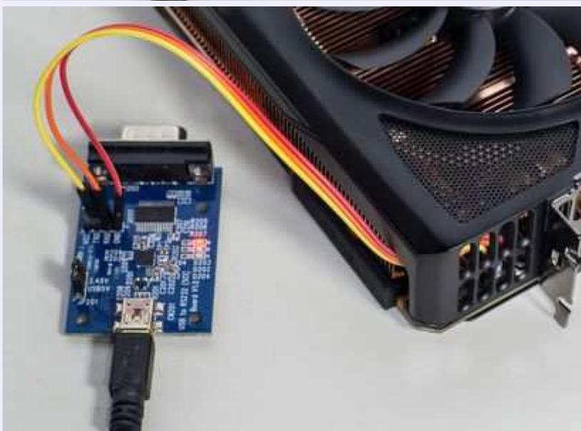
USB end of serial cable goes to your PC or smartphone via OTG, or any other device
